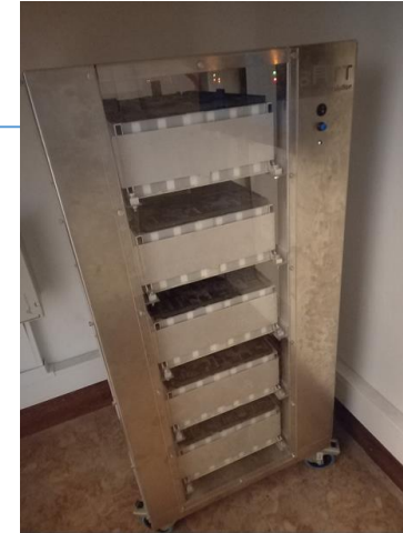
Storage in used EV batteries
